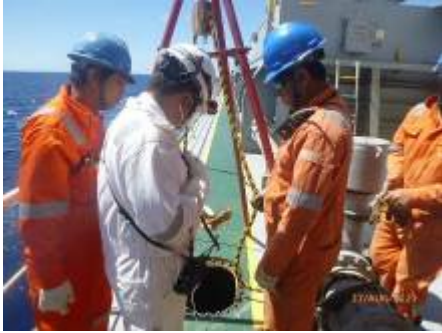
Oxygen and gas content inside the tank measured and found to be safe for entry
